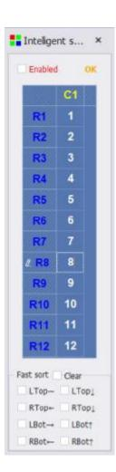
Smart lookup page, you need to check "enable" to take effect, C table column, R represents the row, according to the number displayed on the screen, corresponding to the writing to the software. Quick sort refers to the entry order of 1, which can be quickly sorted by pre-selecting the upper left below and the top right.
