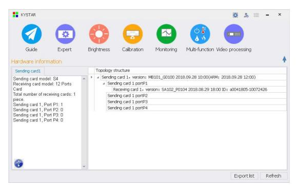
Detecting the device program version can check whether the program version of the sending card and the receiving card is the latest version, and label it with different colors on the topology map: green is the latest program version, and red is not the latest program version.
