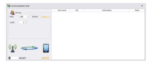
Communication detection can detect the current network cable and receiving card communication status, and can solve the communication problem by replacing the network cable or receiving card in the event of false positives or packet loss.
